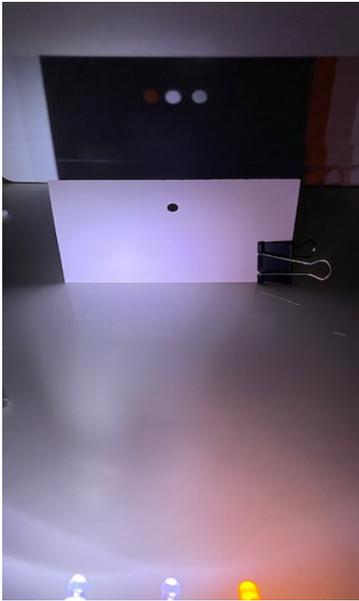
In this photo, the yellowish LED is on the right and an orange-red light dot is on the left. The orange-red color has to do with the mixing of light. This is explained in Colored shadows activity found on our website.
