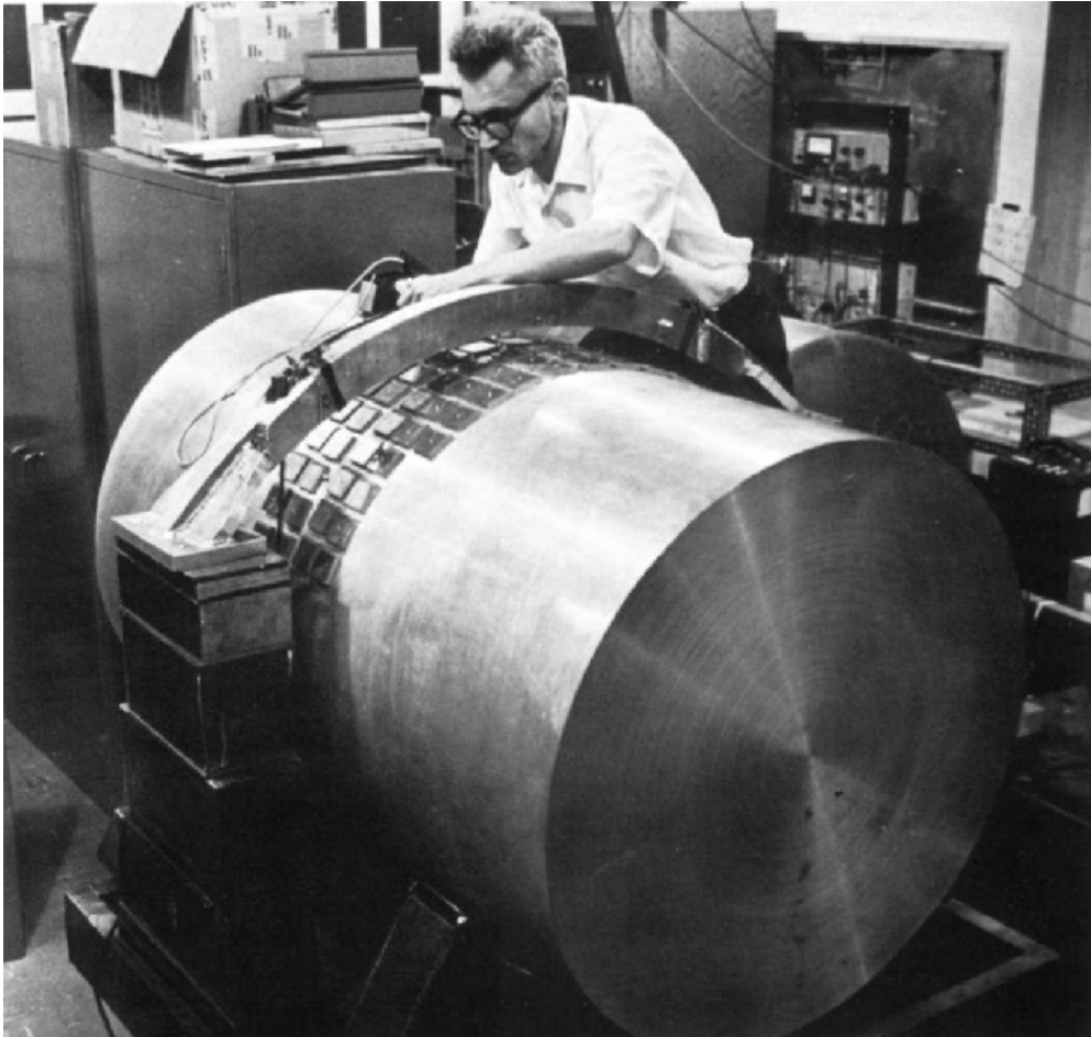
Joe Weber, in 1970, with one of his cylinders suspended on acoustic filters (stacks), at room temperature, with piezos near center
