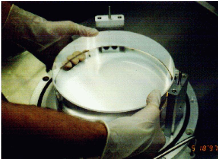
Figure 14: Optic Being Placed In the Carrier
