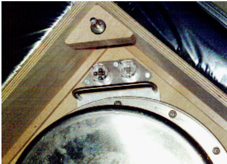
Figure 4: 60g & 150g Shock Indicators
