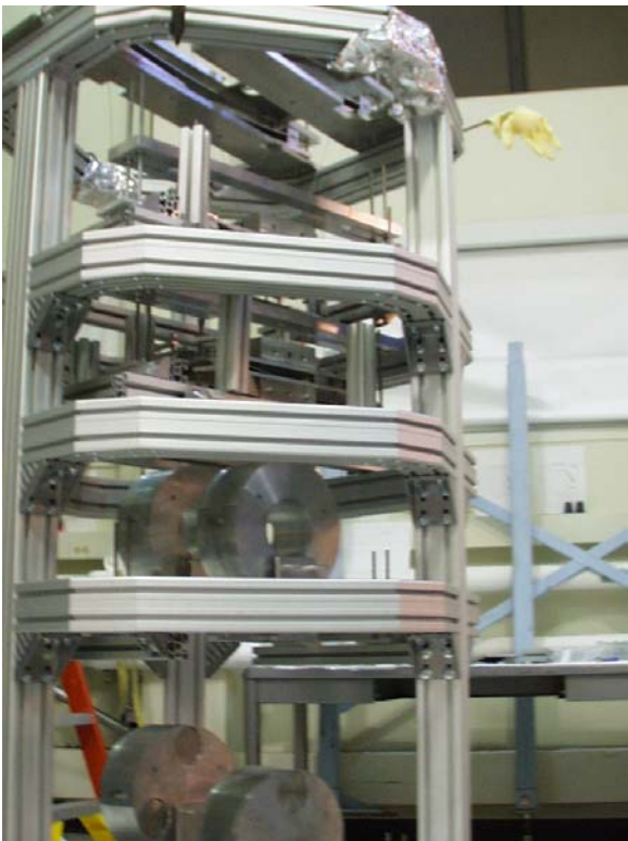
Figure 12. Autocad diagrams and pictures of prototype quadruple pendulum. Top left shows view of quadruple and reaction chain. Crossed blades at top can be seen. Top right shows first two masses in the chain, with the top of the upper mass removed to show where the crossed blades lie within the mass. Bottom left shows assembled pendulum sat MIT. Bottom right shows close up of top masses of both main and reaction chain, with some of local control electronics in place.
