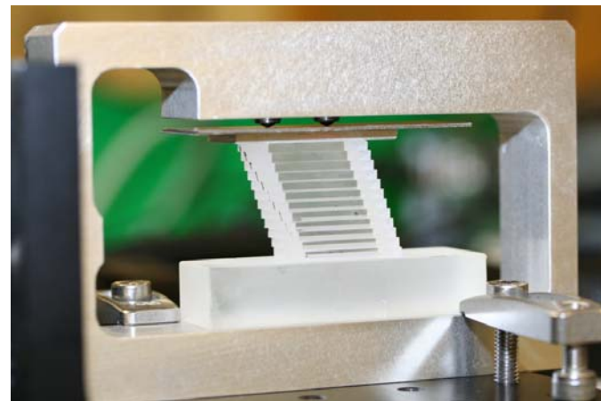
Final prototype slicer unit mounted in measurement setup after bonding, de-bonding and re-bonding
