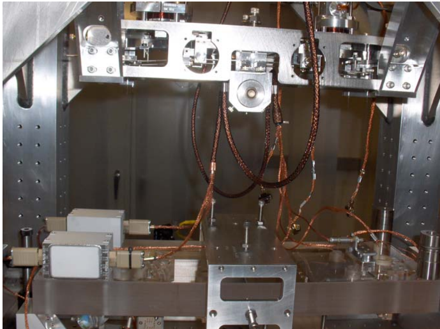
Figure 1 Original concept for wiring of OMC bench. Note the black peek shielding in the upper sections of the two cabling bundles, one bundle from the two preamp boxes on the left and the other from the QPDs etc on the right side.
