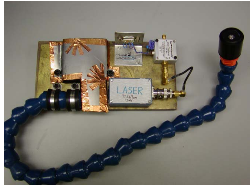
Along the way...AM Laser assembled to test RF Photodiodes, including those in Mode Cleaner Servo
