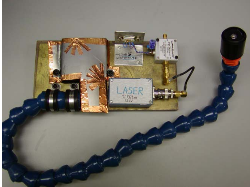
Figure 12: AM Laser. The laser diode is in the box labeled "Laser", and is fiber-coupled. The fiber travels through the blue tubing, and sends the light through a lens at the end of the tube.
