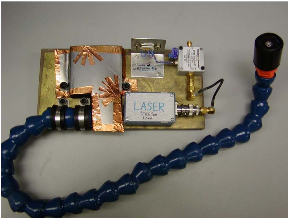
Figure 17: AM laser, fully assembled. A layer of foam and sheet metal has been added to protect the coiled section of fiber.
