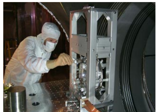
Figure 8 LOS assembly with recycling mirror being adjusted, LHO.
