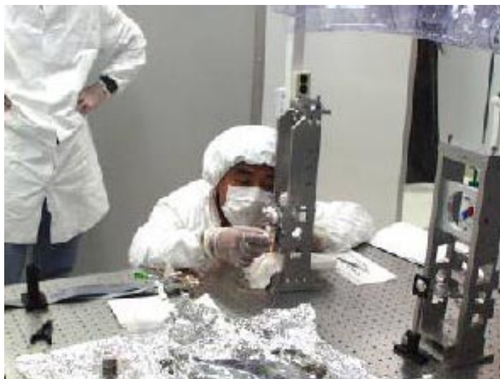
Figure 9 SOS assembly at LHO
