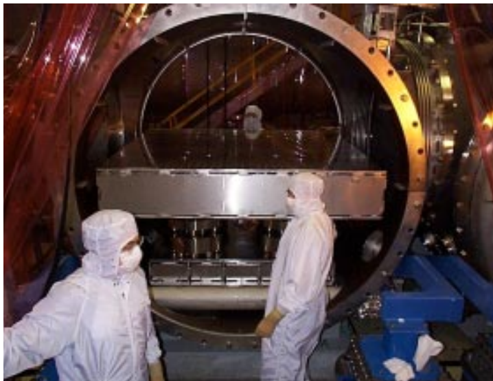
Figure 6 HAM in-vacuum components, LHO
