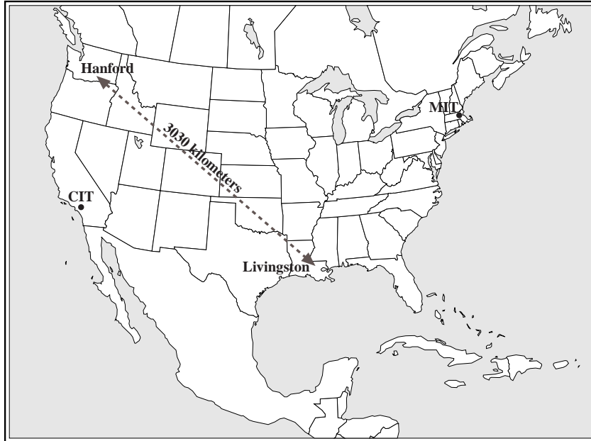
Figure 2: The location of the two LIGO observatories, the sites are separated by a distance of 3030 km, corresponding to a time of arrival difference of \pm 10 ms.
