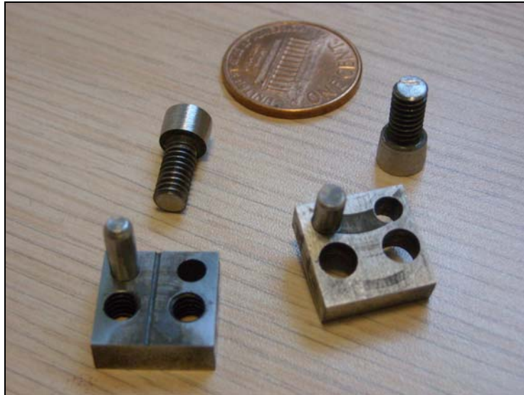
Figure 4-6. The size and layout of the tool steel clamp.
