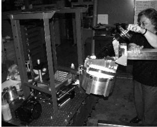
Figure 10. Ergonomic arm being used to manipulate a 40 kg mass in a controlled fashion.
