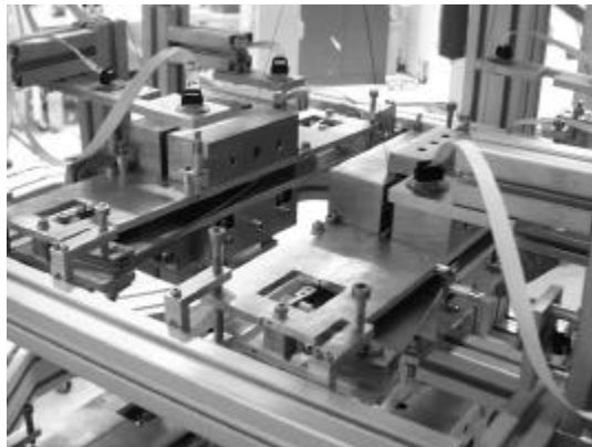
FIG. 8. Two views of the prototype quadruple suspension assembled at MIT. Above is an overall view showing the main and reaction chains, suspended from a support frame. Below is a close-up of the top masses, with some of the local control actuators visible. The construction can be compared to the diagrams in figure 2.
