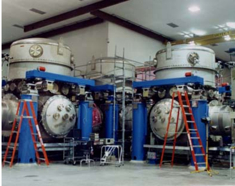
Figure 3. BSCs (Beam Splitter Chambers) in the Corner Station at Livingston
