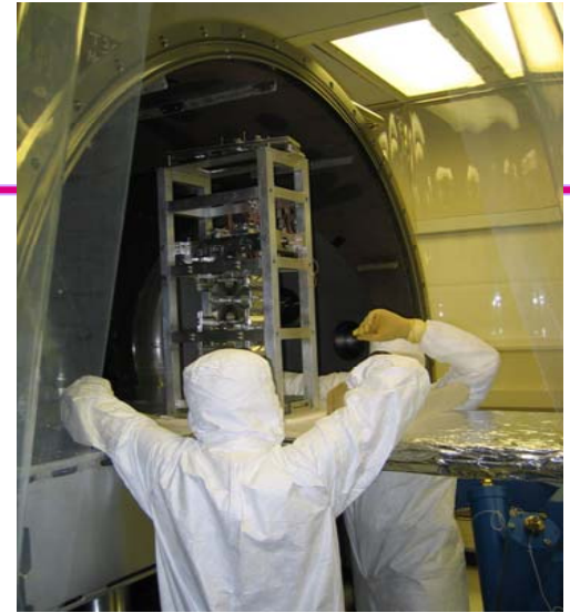
'Controls' Triple Installation at LASTI
