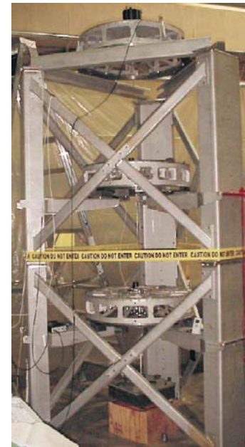
Passive, 'inverted pendulum' and GAS demonstration at CIT
