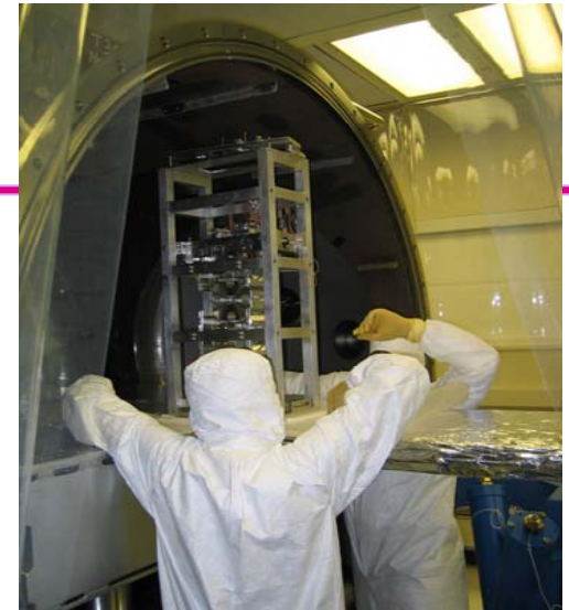
'Controls' Triple Installation at LASTI
